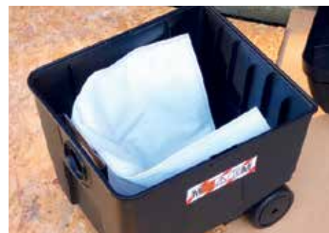
Inside the plastic drum is a disposable fabric collection bag, slotting into a groove just inside the inlet
